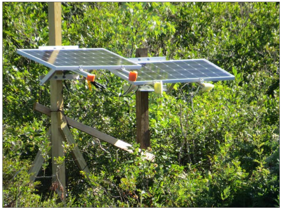
Webcam two was run almost entirely on solar power—the first time LPC has used solar power in our camera setup.
